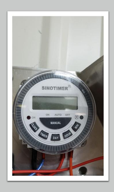
Step 15: Set Clock on digital Timer. Set Timer for Lights to go On and Off. Turn Timer to Auto.
